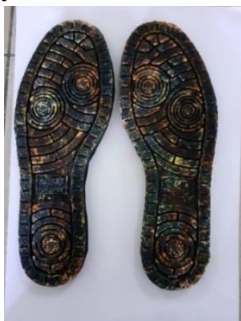
Figure 3. Shoe soles produced with tyre crumbs (GRT) and compounded natural rubber latex
